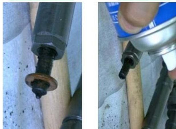
7. Using the SST (E) remove carbon deposits from injector mounting holes (D) in the engine head assembly.
